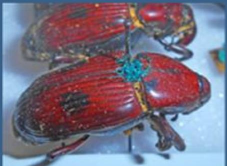
*Verdigris is the result of reactions between atmospheric moisture (humidity), copper, and the chemicals produced by the deterioration of the specimen, or by corrosive vapours and acids emitted by wooden cases or adhesives. Verdigris is blue-green in colour and often has a hair- or thread-like appearance. Verdigris causes discolouration in specimens and can also cause physical damage at the pin site.*
